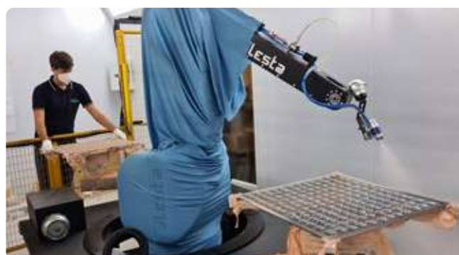
Lesta LEBOT MV A6 on carousel with Easy prog 2D LIQUID OR POWDER APPLICATION FOR SMALL PLASTIC AND METAL COMPONENTS
