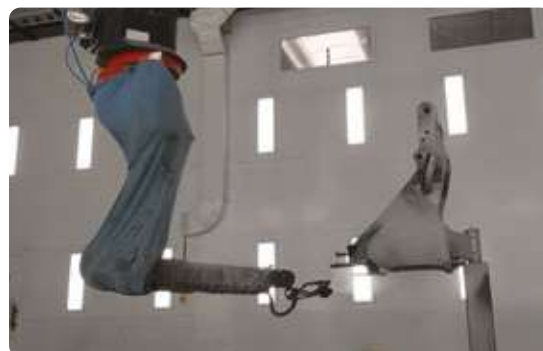
Lesta LEBOT MV A6 on carousel with Easy prog 2D LIQUID OR POWDER APPLICATION FOR SMALL PLASTIC AND METAL COMPONENTS
