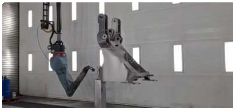
Lesta LEBOT MV A6 on chariot LIQUID APPLICATION FOR METAL
